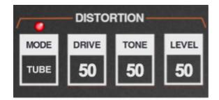
**MODE**- Turns distortion on and off and sets the type. The LED above the MODE button illuminates when distortion is enabled.
