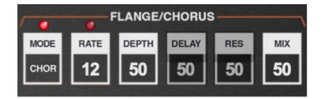
A thick and warm flange/chorus effect. Flanging and Chorus are closely related - the general difference being that flangers use a shorter time range and some amount of feedback (this intensifies the "jet-flyby" whoosh), whereas choruses utilize a slightly longer delay time, and no feedback.
