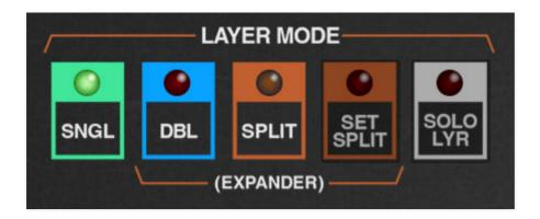
The LAYER MODE section defines overall "single" or "double" behavior as well as configuring splits in DOUBLE mode.
