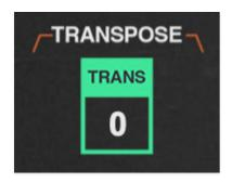
**TRANSPOSE**- The *TRANSPOSE* menu buttons transpose the range of Chroma or Expander up to two octaves up or down. Unlike the PITCH A/B/C/D *RANGE* controls, which only affect one layer at a time, the TRANSPOSE section buttons affect the entire Chroma (A/B) or Expander (C/D) for quick octave changes.
