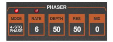
**MODE**- Turns the phaser on and off and sets the phasing type and sync. The LED above the MODE button illuminates when the phaser is enabled.
