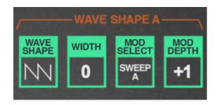
**WAVE SHAPE-** Selects the oscillator waveform. Each oscillator includes triangle, sawtooth, square, variable pulse.
