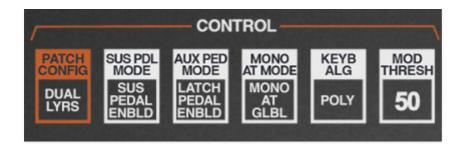
The CONTROL section contains what's often referred to as "global" parameters. Unlike all other PARAMETER PROGRAM controls, these apply to both voice paths - A/B for the Chroma or C/D for the Expander. This is why the word CONTROL (and most of the buttons) is white.
