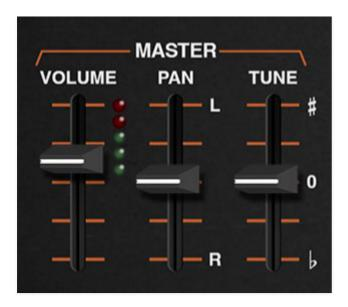
**VOLUME**- Sets the master volume for the entire instrument. The LED meter indicates output level; keep it in the high greens/low red to avoid undesirable digital clipping.
