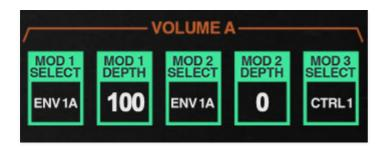
The VOLUME section defines how envelopes generators and other level modulation is applied to shape the amplitude of sounds using a voltage-controlled amplifier (VCA). If you're not familiar with them, think of a VCA as a simple volume knob that gets automatically turned using control voltages.
