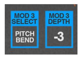
In the PITCH section, locate the mod bus that pitch bend is currently assigned to and invert the MOD DEPTH setting. In the example above, you'd set MOD DEPTH to +3 instead of -3.
