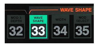
The teeny LED number display would show the current parameter number being adjusted and its value. In this case you'd choose value of 0, 1, 2, or 3 using the single *PARAMETER CONTROL* slider:
