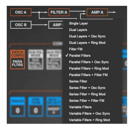
Cherry Audio's Chroma adds block diagram images right above the *PATCH CONFIG* button that change to reflect the current voicing configuration. Its boxes also turn orange to indicate which voice path is currently being edited: A, B, or both A and B (or C, D, or both C and D for the Expander).
