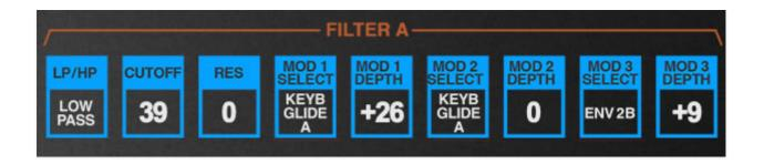
The original Chroma filter made use of CEM3350 chips, which were dual 12 dB/octave state-variable filters ("state-variable" meaning they could be configured as a lowpass filter, a highpass filter, or Maine or Delaware). One "block" in a Chroma voice path equates to a single 12 dB/octave filter which can be set to lowpass or highpass mode. These can be combined to create bandpass or notch filters, or a steeper 24/dB octave slope using Chroma's flexible Patch Configurations.
