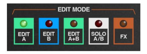
These buttons determine which voice path (or FX section) is currently being edited with the 50 *PARAMETER PROGRAM* controls.
